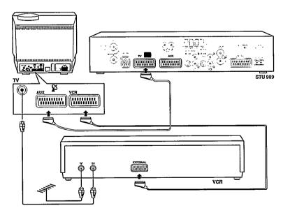
For PHILIPS TV sets with ML, PV or SL in the type number, except for the Wide-Screen 16:9 TV sets, it is recommended to use the connections as shown in the drawing and follow the instructions supplied with the TV set.
